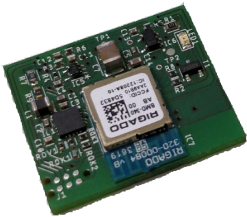
Figure 3: The FLYNC prototype based on the nRF52840. The solar panels on the backside charge a small capacitor that powers the circuit and the MCU.
