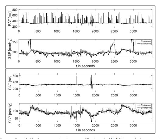
**Figure 5.** Example Blood pressure estimation output (Chen's method [29]) before and after automatic ectopic beat clearance. The pulse arrival time (PAT) trace is given in the top plots, whereas the continuous systolic blood pressure (SBP) reference along with the estimated SBP (bold) are plotted at the bottom.
