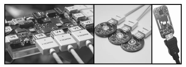
**Figure 2.** Assembled hardware system: (a) ECG sensor mainboard; (b) active ECG electrodes; and the (c) PPG module for acquiring the optical pulse wave signal.
